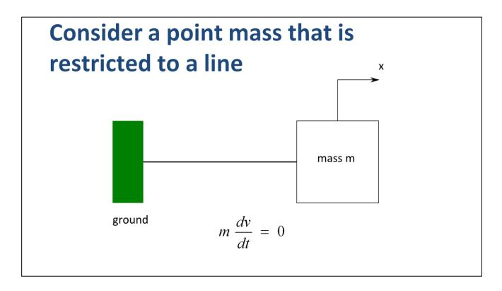
First we start with our mass that is free to move along the x-axis. There are no forces so the acceleration is zero.
