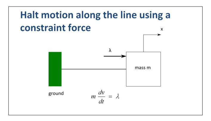
Now we bring in a constraint force lambda that acts along the x-axis. The job of this constraint is to halt motion along the x-axis.
