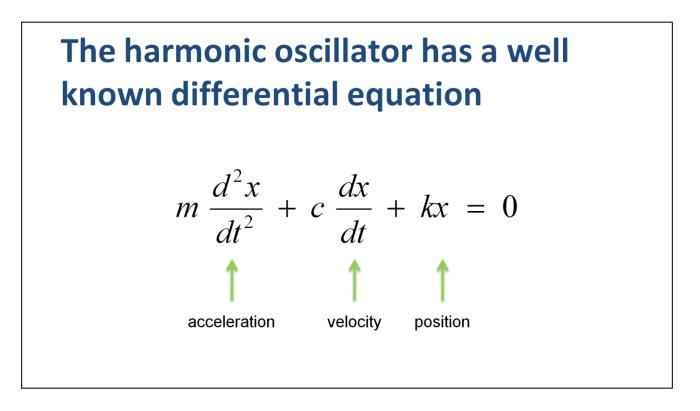
To understand how the harmonic oscillator moves, we need its differential equation. Here we have the well known equation of motion for the harmonic oscillator, which is just an expression of Newton's law, force equals mass times acceleration. In this case the spring and damper are the forces.
