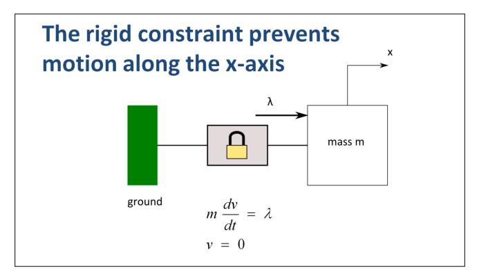
The constraint force seeks to keep the x-axis velocity at zero.
