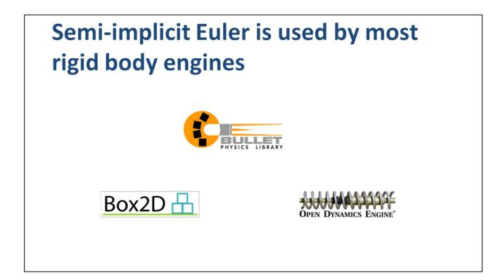
Semi-implicit Euler is the integrator of choice for most physics engines. It is cheap, stable, and works well with rigid body constraints. In fact, most modern constraint solvers are designed to work with semi-implicit Euler.
